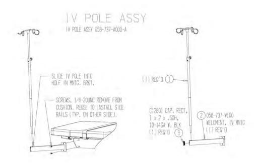
Figure 14. Installing the I.V. pole.
