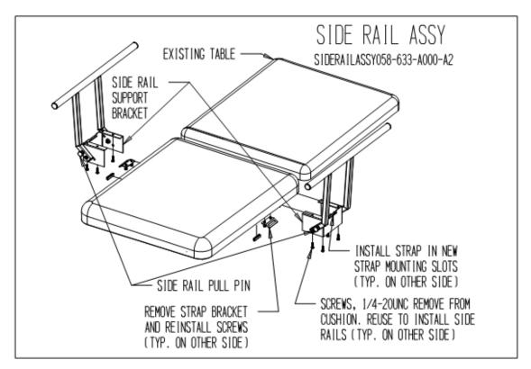
Figure 9. Installing the side rails.
